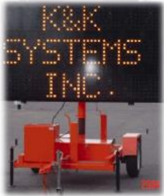
Figure 157-30 Portable LED sign (prohibited)
